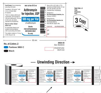
This Eye Mark should be at back sideon release liner (in between two labels) to sense the label on machine
